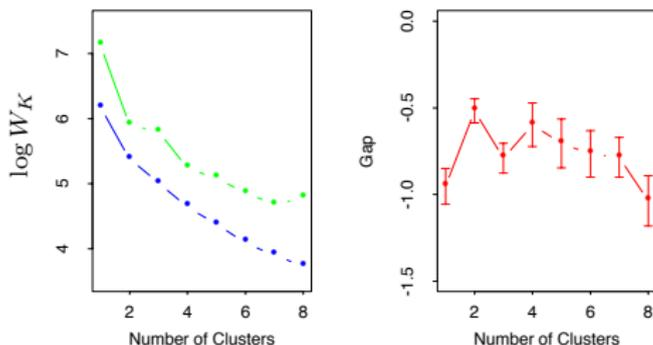
Figure 14.11: *Left panel: observed (green) and expected (blue) values of  $\log W_K$  for the simulated data of Figure 14.4. Right panel: Gap curve, equal to the difference between the observed and expected values of  $\log W_K$ . The Gap estimate  $K^*$  is the smallest  $K$  producing a gap within one standard deviation of the maximum; here  $K^* = 2$ .*
